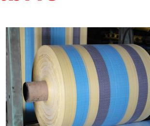
Woven fabric is obtained when the cloth is woven and are made in a set of two different fibers. One of the fiber in the woven fabric goes in the direction of the length of fabric while the other one
